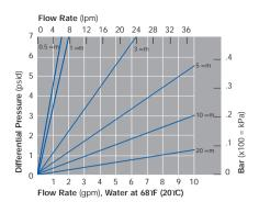
Flow rate is per 10" (25.4 cm) cartridge. For liquids other than water, multiply differential pressure by fluid viscosity (CP).
